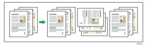
To use the Rotate Sort function, two paper trays loaded with paper of the same size and type, but in different orientation ( $\square\square$ ), are required. For details, see "Tray Paper Settings", Connecting the Machine/System Settings.
