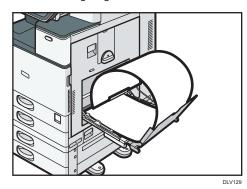
• When using paper that has a horizontal width of 900 mm (35.5 inches), curl the paper so
