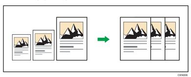
• If you select a reproduction ratio after pressing [Auto Reduce / Enlarge], [Auto Reduce / Enlarge] is canceled and the image cannot be rotated automatically.
